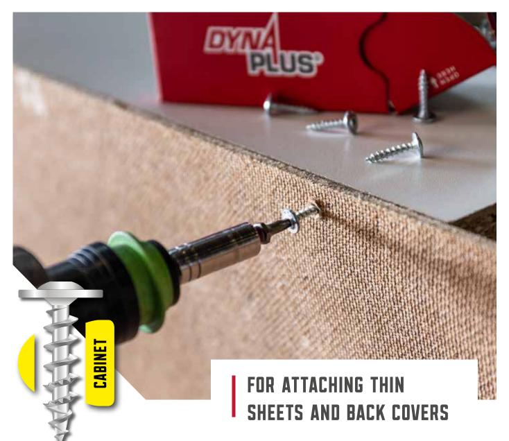
Dynaplus® cabinet screws are specifically developed for attaching thin sheets and back covers to cabinets and kitchen cupboards. The large head with fused washer provides for an extra large clamping surface which enables you to firmly attach the back cover.
