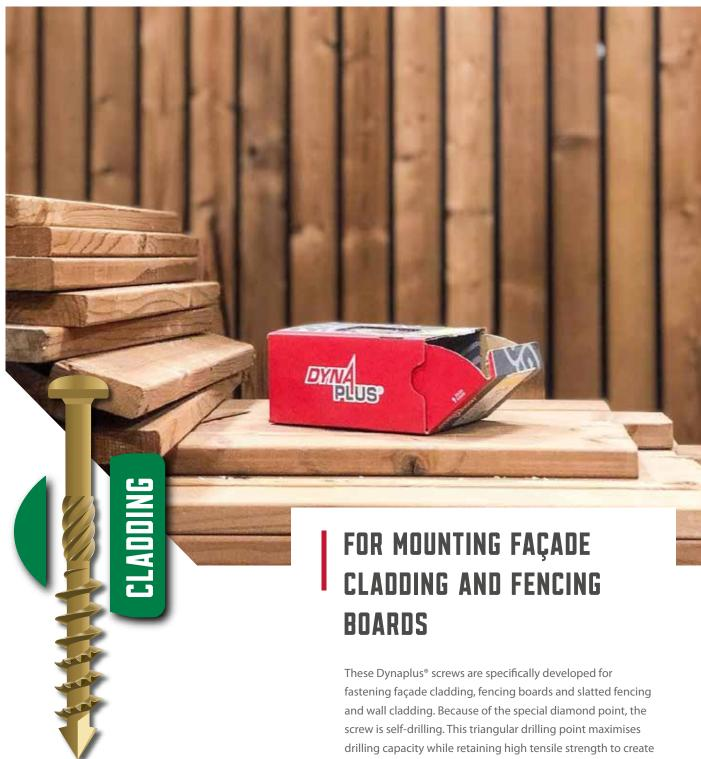
a solid connection. As a result you can drive in the screws up to two centimetres from the edge of the board without predrilling and without splitting the wood.
