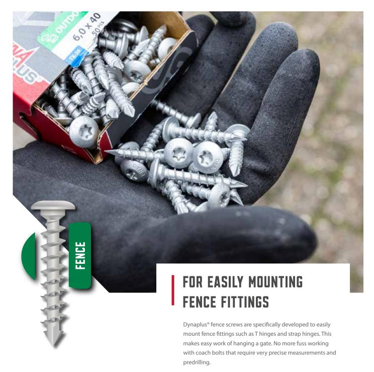
The fence screws make it easy for you to hang your garden gate. These strong screws are made of hardened carbon steel and are protected against corrosion by the silver-grey anti-rust (AR) coating. This coating falls in the highest RISE corrosivity class: C4, and consists of three thin organic layers applied on top of the galvanised zinc layer which provides for excellent adhesion.
